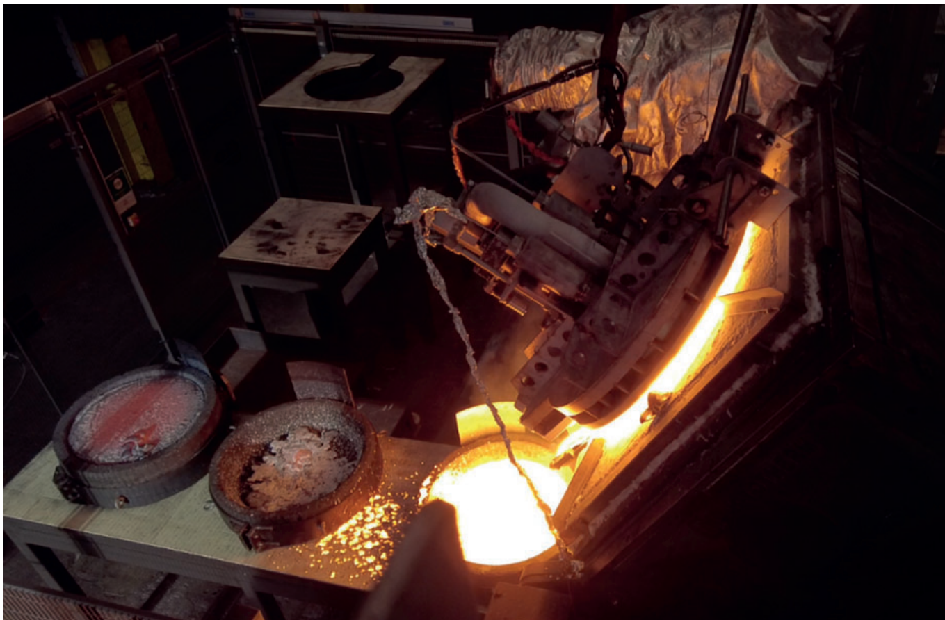
Casting of SisAl slag at Elkem pilot
