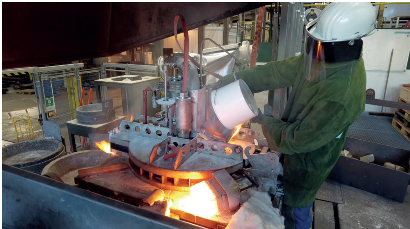
Charging of raw materials to the induction furnace at Elkem
