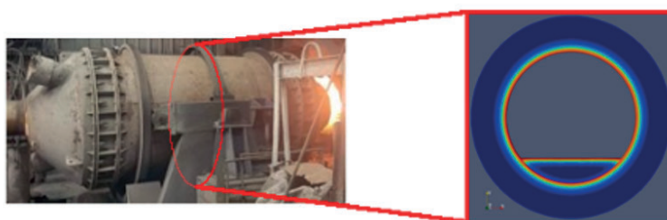
Distribution of temperatures in the FRey rotary furnace.
